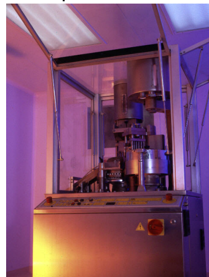
One of our two 40,000 capsules per hour automatic encapsulating machines
